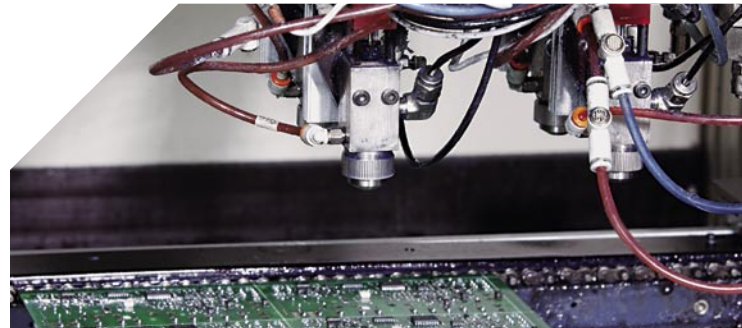
In-line conformal coating and encapsulation of circuitry.
